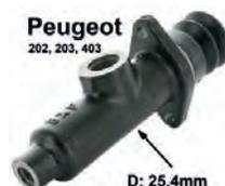
P 202/203/403, Hauptbremszylinder Peugeot 202, Peugeot 203, Peugeot 403. Kolben 25,4mm. (1 Zoll). Original Lieferant!
