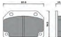
Talbot Horizon, Rancho, Bremsklötze. Breite 83,7mm, Höhe 55mm, Dicke 15mm.
