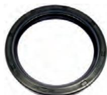
Simmerring Kurbelwelle hinten. Abmessung: 80 x 100 x 13mm. Passend für R4 (955, 956, 1108ccm), R5, Estafette, R12, Fuego, R11, R20, R30, R25, R16, R15. Peugeot 504 V6, 604 V6, Citroen XM V6. Made in Germany.
