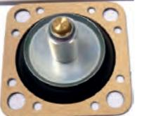
Membrane Beschleunigerpumpe, Peugeot 104 + 205 Solex 32 BIS + 32 PBISA 7-8-11. Citroën Visa, BX, AX Solex 32 PBISA 7-8-11-12-16 + 34/34 Z1. Renault R5, R9, R11, R14 32 BIS + 32 PBISA. Talbot Samba + Horizon 35 BISA8 + 32 BIS. Stößelhöhe 14,5mm.
