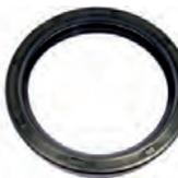
Simmerring Kurbelwelle hinten. Abmessung: 80 x 100 x 13mm. Passend für R4 (955, 956, 1108ccm), R5, Estafette, R12, Fuego, R11, R20, R30, R25, R16, R15. Peugeot 504 V6, 604 V6, Citroën XM V6. Made in Germany.
