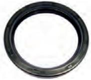
Simmerring Kurbelwelle hinten. Abmessung: 80 x 100 x 13mm. Passend für R4 (955, 956, 1108ccm), R5, Estafette, R12, Fuego, R11, R20, R30, R25, R16, R15. Peugeot 504 V6, 604 V6, Citroën XM V6. Made in Germany.
