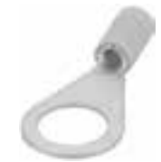
Eye ring yellow, 12mm attaching lug. Yellow = cable diameter: 3,6 to 6,8mm.
