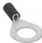
Eye ring blue, 10mm attaching lug. Blue = cable diameter: 2,3 to 5,0mm.
