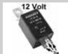
Flashing relay, 12 V, 3 plug connections. 2x 21 Watt power output. Suitable for Citroën 2CV, DS, HY, Renault R4, Peugeot 203, 403, 404 etc. Connection French: Current supply symbol (+). Connection indicator in front + rear = symbol (C). Connection control light dashboard = symbol (R). If a Japanese relay is used: Plus + = symbol X or B. Connection indicator C = symbol L. connection control of R = symbol P.
