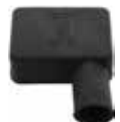
Battery pole protecting cap from rubber. Color: black. Length: 52mm. Wide one: 35mm. Long side left - cable inlet down.
