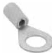
Eye ring yellow, 10mm attaching lug. Yellow = cable diameter: 3,6 to 6,8mm.
