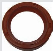
Shaft seal crankshaft in front, for Citroen 2CV (all engines). Improved version from silicone. Measurement: 30x42x8mm
