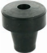
Bumpers rubber buffers, for Citroen 2CV. This rubber is rear, mounted from above onto the front bumpers. It is the base for the bonnet! Often this rubber is missing, and the bonnet rubs on the bumper.
