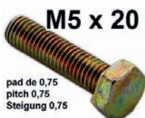
M5x20, pitch 0,75! Screw yellow chromated. Note: This screw has a 0.75 pitch, as it was originally installed from Citroen, at the beginning of the seventies. Today's screws have 0,80 pitch !
