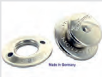
Loxx, snap fastener, upper part, on textile. Very simple and clever system, german invention from 1928. It works like a trailer coupling. The upper part catches a small ball and the system is locked. To open just pull up the upper part. No more broken fingernails! Just perfect.
