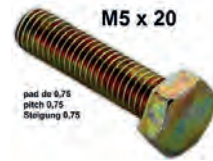
M5x20, pitch 0,75! Screw yellow chromated. Note: This screw has a 0.75 pitch, as it was originally installed from Citroën, at the beginning of the seventies (S.i.m). Today's screws have 0,80 pitch! (ISO)
