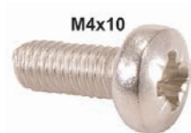
Cross lens head screw (M4x10) from stainless steel, for round indicator + stop light. For Seima + AXO caps. Only suitable for metal bases. Per piece
