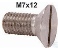
M7x12. Countersunk screw 7mm, with flat bolt head! Material: High-grade steel. The bolt head has about 12mm diameter! E.G. suitable for the door lock wedges (Citroën 11CV).
